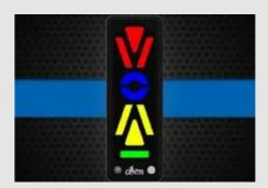
The photo above shows an AoA indicator for a general aviation aircraft. I have such a system in my own aircraft and it can be a life saver in critical situations.
