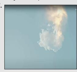
The vehicle experienced multiple engines out during the flight test, lost explosion. altitude, and began to tumble. The flight termination system was commanded on both the booster and ship. As is standard procedure, the pad and surrounding
