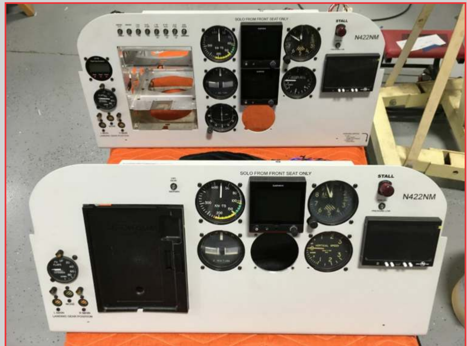
Photo below: New instrument panels designed, fabricated, painted, laser engraved, assembled
