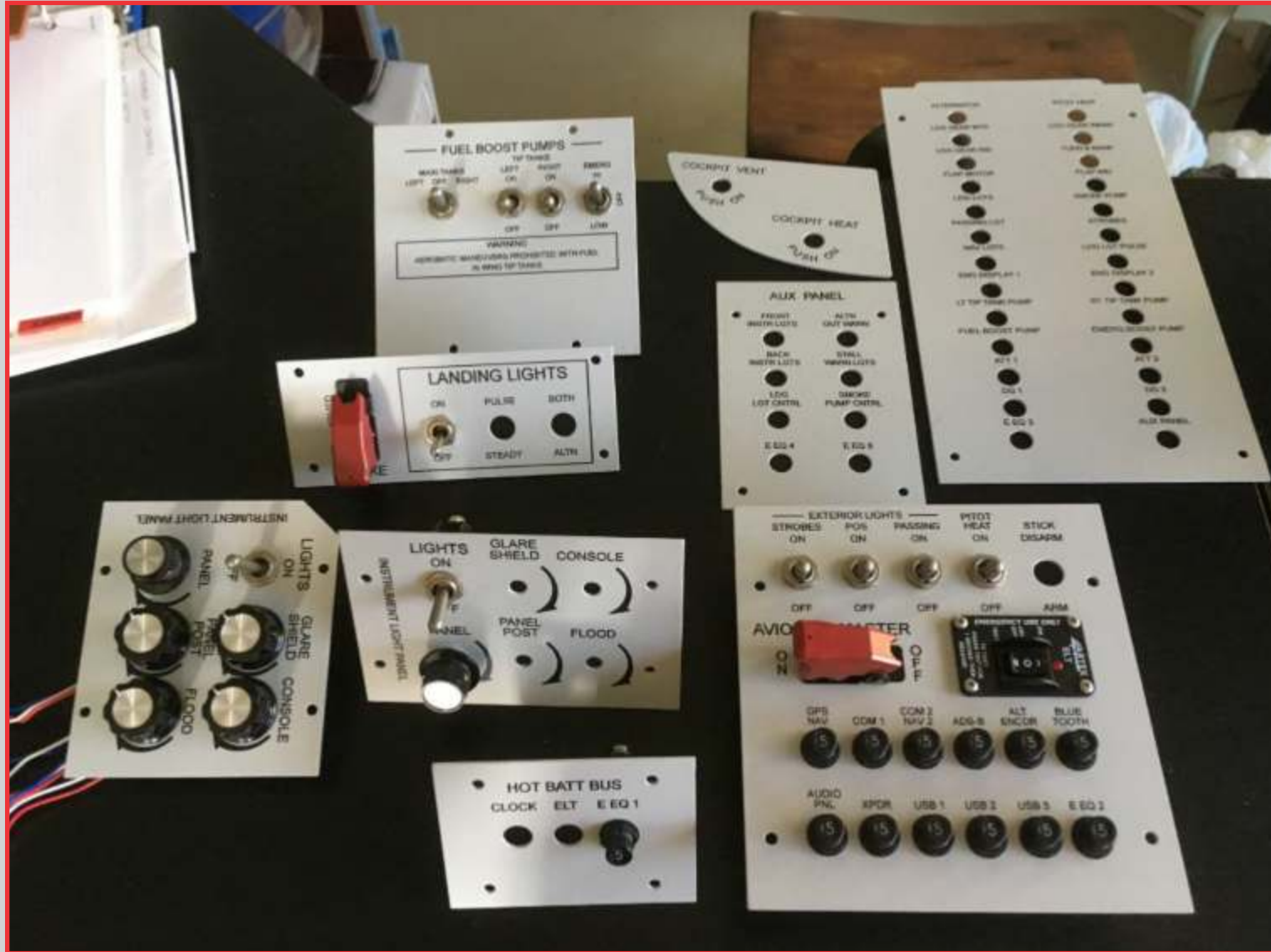
Photo above: New sub-panel pieces designed, fabricated, painted, laser engraved
