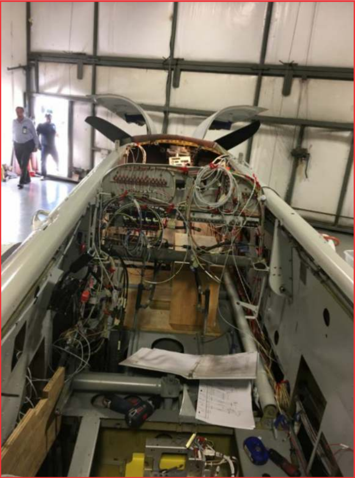
Photo below: Cockpits disassembled, new wiring/upgrades in-progress
