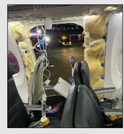
Fortunately the plane was at a relatively low altitude of 16000 ft when this major incident took place. As a result it quickly descended to below 10000 ft which is the height below which hypoxia is not a major issue. However, the oxygen masks appear to have deployed correctly.
