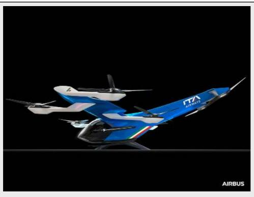
and eight electrically powered propellers as part of its uniquely designed distributed propulsion four passengers - including a pilot in zero-emission flights for multiple such as the development of urban applications. CityAirbus NextGen is being developed to fly with a 80 km operational range and to reach a 28 aircraft from the manufacturer, cruise speed of 120 km/h, making it including seven A220s, 11 perfectly suited for a variety of missions.
